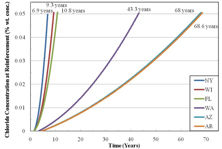
Time to corrosion initiation for RC
